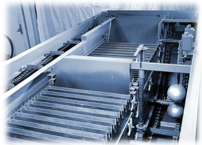
SEP features an automated conveyor-aided filtration system-removes chips and fines with minimal maintenance
